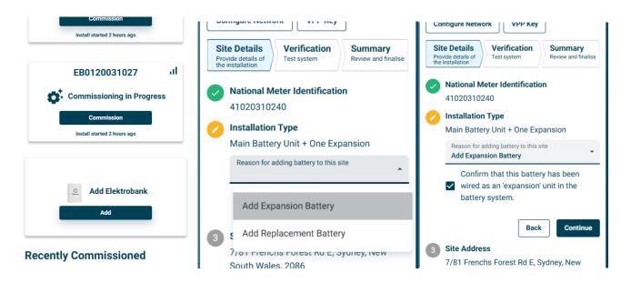
5. Carry out all necessary tests for the expansion unit. Once these tests have been successfully completed, click the 'Continue Setup' link to proceed with testing the main unit and finalising site commissioning—unless you need to add more expansion units, in which case, repeat the process for each additional unit before continuing.
