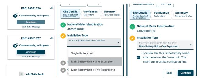
3. After entering all the site and installation details for the 'main' unit, complete all tests for the 'main' unit up until a final 'Multi-Battery (Stack) Disconnect Verification' test which will prompt that expansion units must be configured before continuing:
