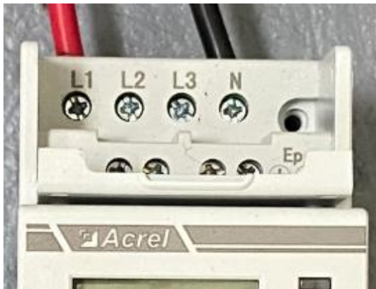
Figure 22: ADL400N showing L1 and N Wired (single phase)
