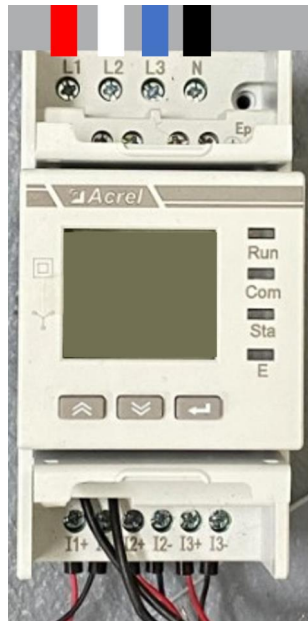
Figure 27: ADL400N wired for 3-phase
