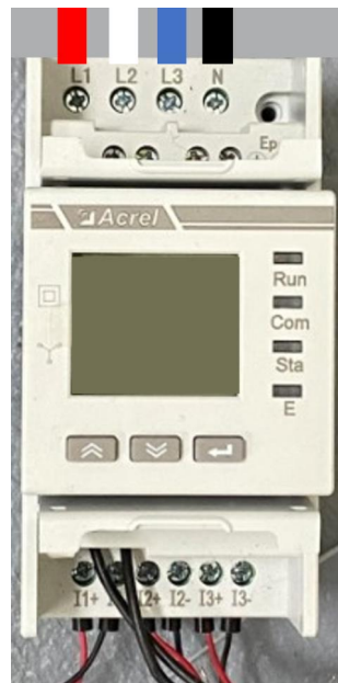
Figure 27: ADL400N wired for 3-phase
