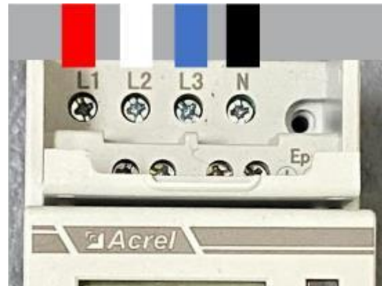
Figure 23: ADL400N showing L1, L2, L3 and N Wired (3-phase)
