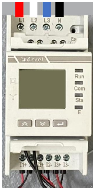
Figure 27: ADL400N wired for 3-phase
