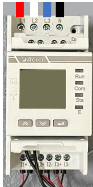
Figure 27: ADL400N wired for 3-phase
