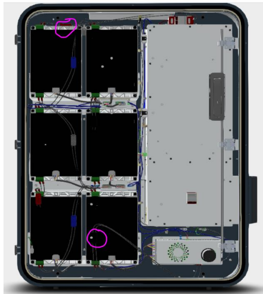
Figure 8 - Battery Stack Connections
